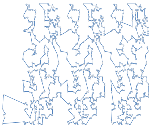
Fig. 3. Example of the pr1002 problem with application of Wang’s Neural Network with Soft WTA and ACO principles: cost of 266118 and average error of 2.73%.
